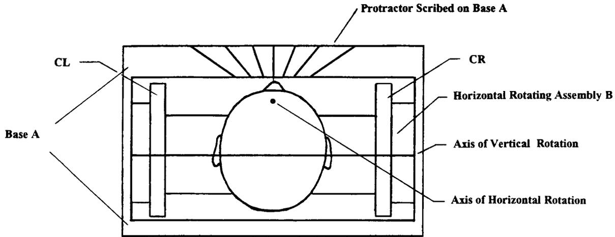
FIG. 4 Top View Showing Base for Horizontal Rotation
