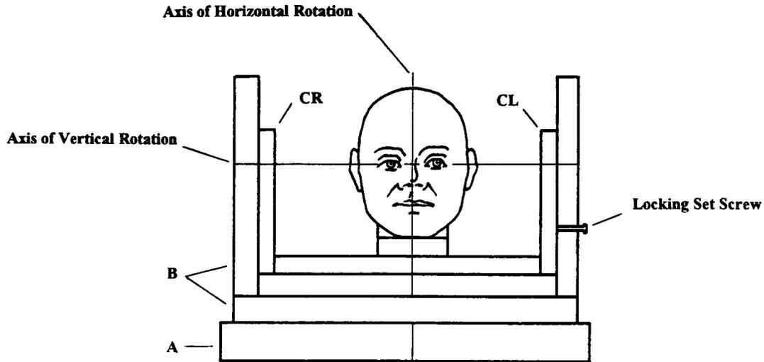
FIG. 2 Schematic of Gimbal for Supporting Standard Head
