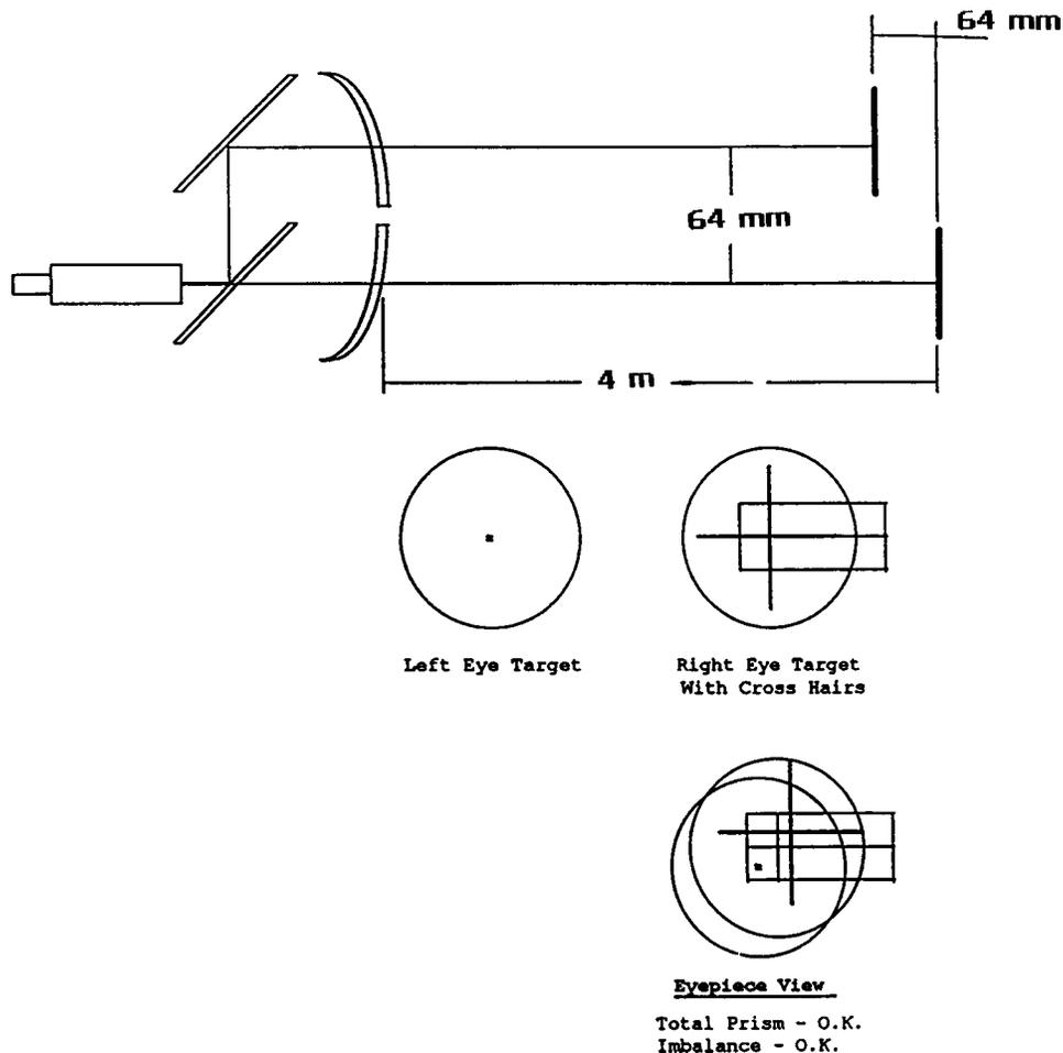
FIG. 6 Alternate Prism Test Set-Up (See 6.8.1)
